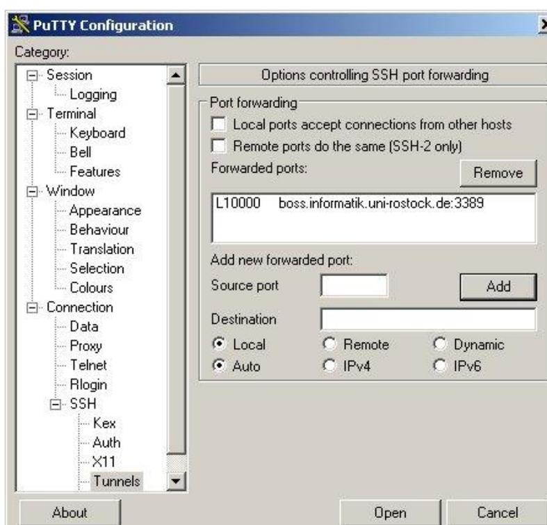
Figure 3 State after tunnel configuration
